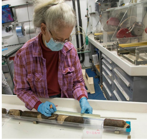
Pamela draws the splitting lines on the core
