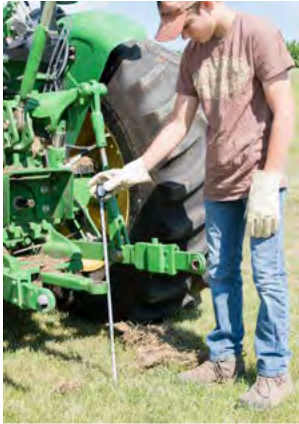
Figure 5.1.d. Tractor drawbars are designed at the correct height from the ground to keep the pull forces below the center of gravity. Credit: Jeff Mathison
