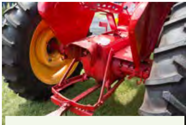
Figure 4.2.c. Power take-off stub and PTO shaft must be properly guarded to prevent entanglements. Locate the PTO area on every tractor you operate. Check whether or not that area is safely guarded. Credit: Michael Houtz, Penn State
