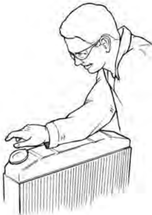
Figure 4.4.f. Wait until the engine is cool to remove the radiator cap. Illustration by Andy Mylin
