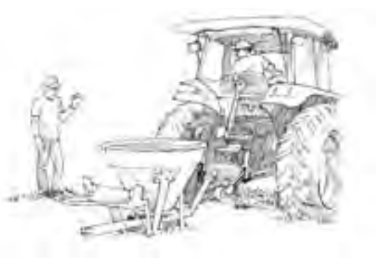
Figure 5.3.b. When connecting drawbar implements, never let a helper stand between the tractor and three-point hitch implement. Crushing injuries and death can result. Illustration by Jeff Mathison
