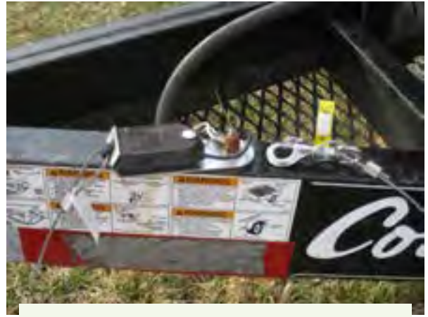
Figure 6.6.c. Surge brakes assist in braking capacity and are activated when the tow vehicle slows down. The trailer pushes against the mechanism in the trailer hitch, causing pressure on the trailer brakes. There is a cable coming out of the hitch that is connected to the tow point and a break away switch in the trailer hitch. Be sure the cable for these brakes is connected to the bumper of the tow vehicle. Credit: Penn State Extension Ag Safety Team
