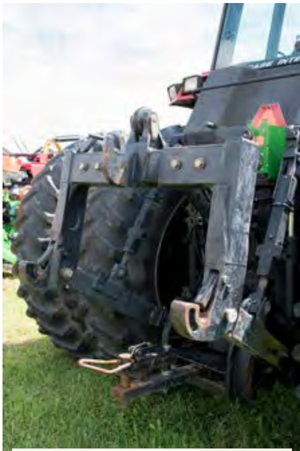
Figure 5.1.h. Heavy-duty quick-attach couplers are mounted on to the tractor's three-point hitch and can safely handle large three-point hitch implements without a person moving between the tractor and the implement. Refer to the owner's manual for additional instructions on their use or have a qualified operator demonstrate the correct procedure for using a quick-attach coupler. Credit: Jeff Mathison
