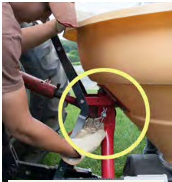
Figure 5.3.d. After adjusting the upper link of the tractor's three-point hitch to align with the upper hitch point of the implement, secure the equipment with the proper size hitch pin and security clip. The circled area indicates where the upper link may be adjusted for fit. The implement must be in a level position after the connection is made. (see Task Sheet 5.2). Credit: Jeff Mathison
