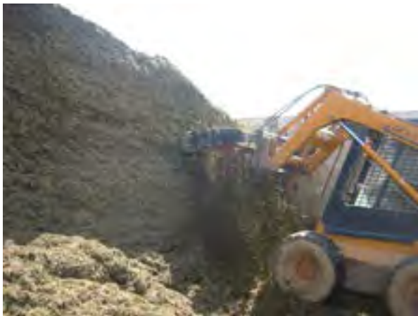
Figure 3.9.1.g. A silage defacer mounted on a skid steer can reach the top of the silage face, but a material handler with a boom may be needed to remove silage from higher reaches. Credit: Penn State Extension Ag Safety Team
