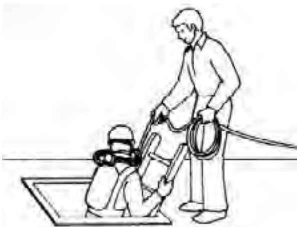
Figure 3.11.d. Only trained person using a self-contained breathing apparatus should enter a manure pit. A lifeline is also a part of safe entry. Do not work alone. Credit: Penn State Extension Ag Safety Team
