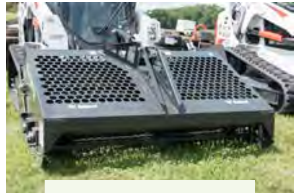
Figure 6.1.3.c. A hydraulically operated tiller attachment is shown. Credit: Jeff Mathison
