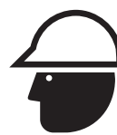
Figure 2.10.g. When you see this symbol, hard hats are required for head protection. Credit: AEM Pictorial Database
