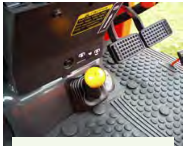
Figure 4.5.3.a. Yellow color-coded controls engage accessories. This is often done through the PTO. Credit: Penn State Extension Ag Safety Team
