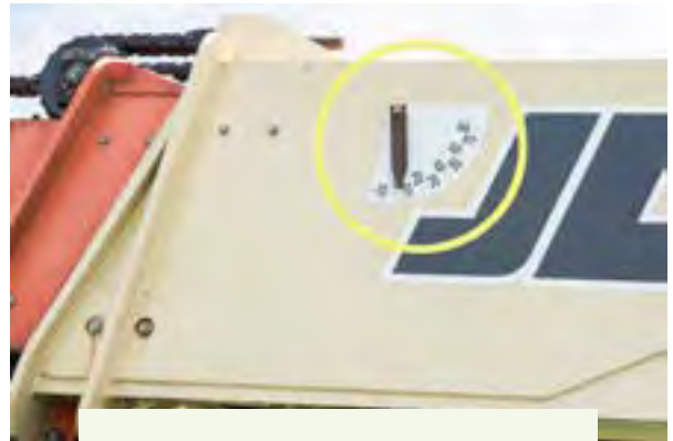
Figure 6.3.f. A typical boom angle indicator is visible to the operator from the cab seat. A similar indicator is found on the instrument panel to show frame angle. Credit: Jeff Mathison
