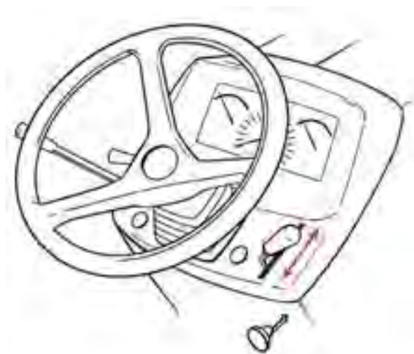
Figure 4.7.c. Set the throttle to 1/3 of the working range. Illustration by Andy Mylin
