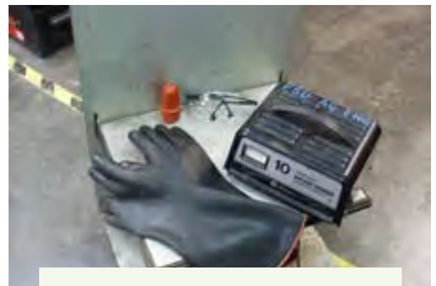
Figure 4.6.3b. Tools you will need to change a battery. Credit: Penn State Extension Ag Safety Team
