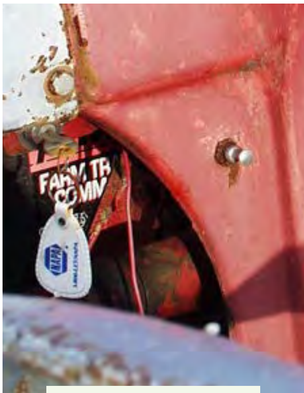
Figure 4.5.1.c. Key switch on lower left of older tractor. Credit: Penn State Extension Ag Safety Team
