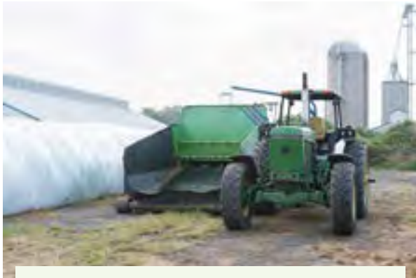
Figure 6.9.a. Silage bagging equipment is driven by the PTO of the bagging tractor. A second tractor or dump truck and unloading equipment is operated in close proximity to the tractor and bagging equipment and must be moved slowly forward as the bag is filled. Credit: Jeff Mathison
