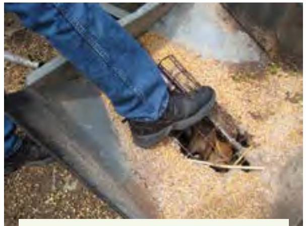
Figure 6.7.a. Augers are found in many places. Augers move grain and feedstuffs into bins and processors and carry these materials to feed carts, grinders-mixers, and feed bunks. The moving parts can pull a user into the machine. Augers should be guarded as shown. Auger guards must be kept in safe condition. The picture shows how effective the guard can be at protecting the user. Credit: Penn State Extension Ag Safety Team
