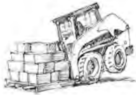
Figure 6.1.c. Skid steer loaders can tip forward if overloaded. This is an important reason to wear the seat belt and understand the skid loader's load limitations. Illustration by Jeff Mathison
