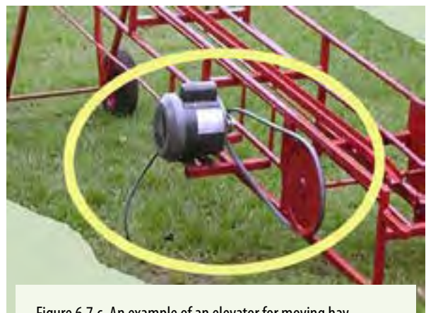
Figure 6.7.c. An example of an elevator for moving hay. Note the turning parts (motor pulley, belt, and drive pulley) as well as the open frame structure. Homemade elevators may be made with solid wooden sides and bottom. Because of the unguarded pulleys and belt, this is an unsafe drive mechanism. Credit for images: Jeff Mathison
