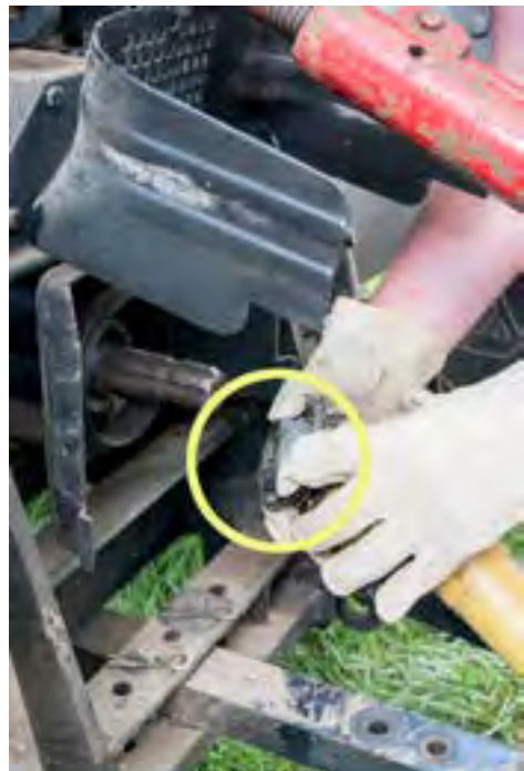
Figure 5.4.e. The sliding collar lock on the PTO driveline has a metal collar that retracts. When the collar is released, springs force the collar forward and secure locking pins in the PTO stub shaft groove to secure it. A firm grip is needed to slide the collar. Credit: Jeff Mathison
