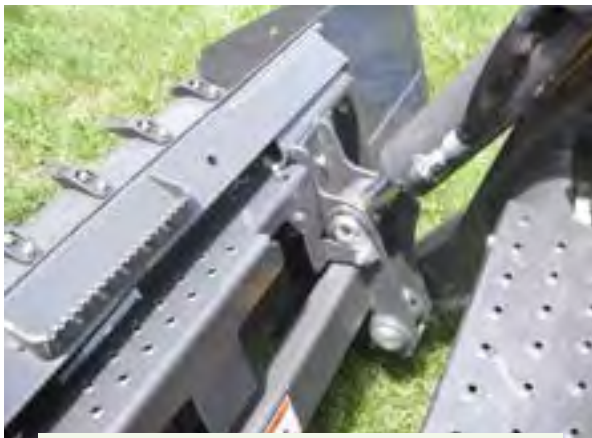
Figure 6.1.3.b. If the skid steer loader mounting plate does not have latch handles to lock the attachment, look for the hydraulically operated pins that provide the locking mechanism and the hydraulic control that activates the lock pin. Credit: Jeff Mathison
