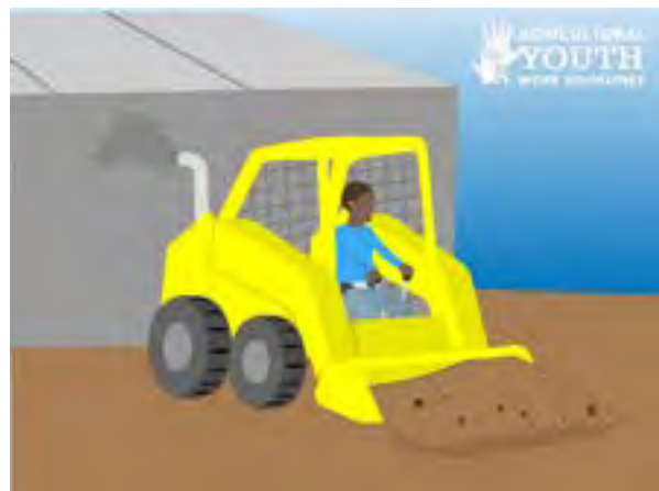
Figure 6.1.a. Skid steers are controlled by hand levers or joy sticks. Push the levers forward to travel forward; pull back to go in reverse. Let go to stop. The levers also steer the machine. Credit: Agricultural Youth Work Guidelines
