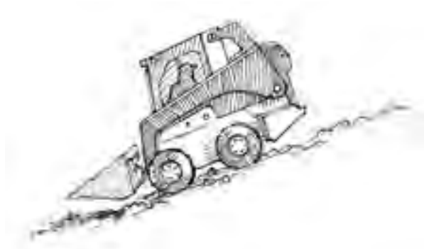
Figure 6.1.d. With no load in the bucket, the safest practice is to back up a steep slope. With a loaded bucket, drive up a steep slope with the bucket lowered. Illustration by Jeff Mathison
