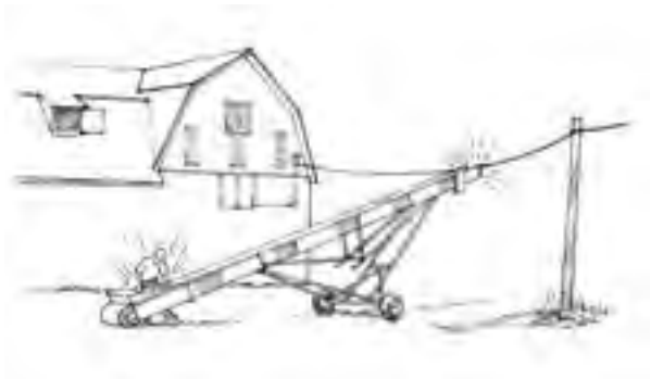
Figure 6.7.e. There is an increased risk of contacting overhead power lines when the auger or elevator is not lowered for transport. Illustration by Jeff Mathison
