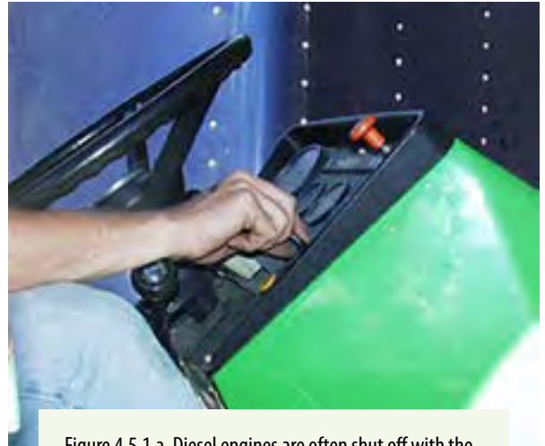
Figure 4.5.1.a. Diesel engines are often shut off with the fuel shutoff switch, not the ignition key. Credit: Penn State Extension Ag Safety Team
