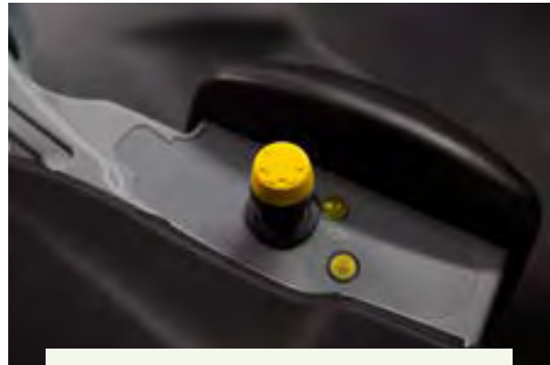
Figure 4.5.5.a.(b). Power take-off (PTO) control, interior. Credit: Michael Houtz, Penn State
