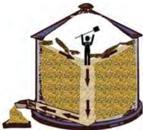
Figure 3.10.e. As the grain bridge gives way, the worker is pulled into the pocket and engulfed. The grain auger may have been left running and the flowing grain pulls the victim under the grain. Credit: Penn State Extension Ag Safety Team
