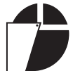
Figure 2.10.c. Face shields are recommended when you see this symbol. Credit: AEM Pictorial Database
