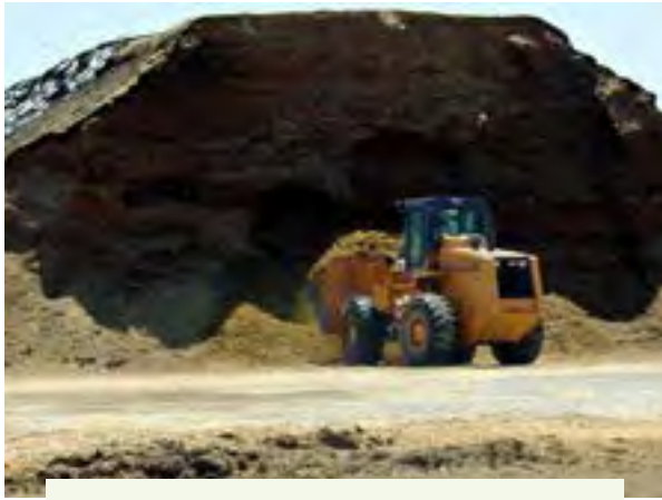
Figure 3.9.1.f. Equipment that cannot reach to the top of the silage face will undercut the feed-out face at the bottom. A collapse of the silage can result. Credit: Courtesy of K. J. Bolsen
