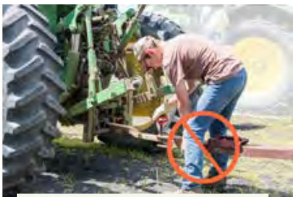
Figure 5.2.b. If you need help hitching to a machine, insist that the helper stand off to the side of the operation. Many people have been crushed between tractors and machines while trying to help connect the machine to the tractor. This picture shows an unsafe act. Credit: Jeff Mathison
