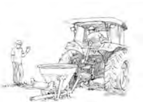
Figure 5.1.g. Never let another person stand between the tractor and the implement during hitching. Too fast of an approach or the operator's foot slipping from the clutch can lead to injury or fatality to the person standing nearby. Illustration by Jeff Mathison
