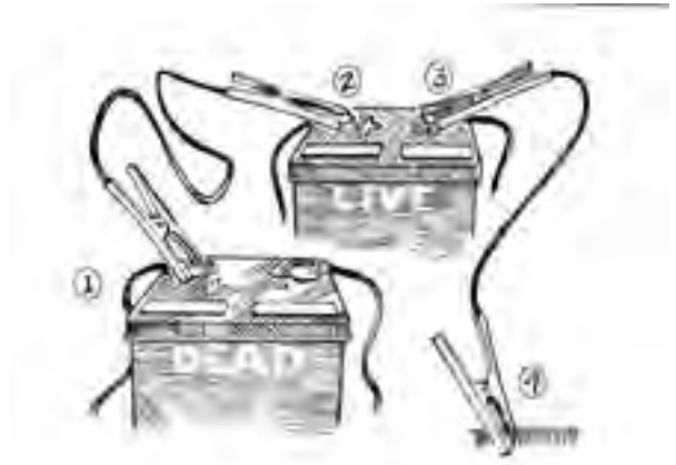
Figure 4.6.4.a. Battery polarity. A battery has two poles or posts. The positive battery post is usually marked POS, P, or (+ or red) and is larger than the negative post, which is usually marked NEG, N, or (- or black). Illustration by Jeff Mathison
