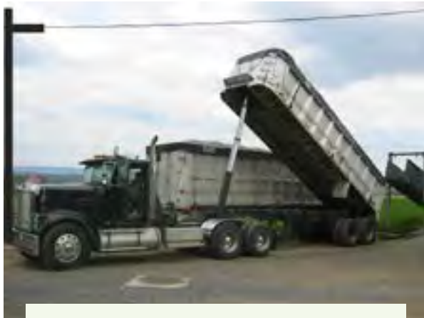
Figure 6.5.d. A hydraulic lift cylinder raises the dump bed to unload materials. As the dump truck or trailer bed is raised, the center of gravity is also raised. When unloading, park the truck on a level, firm surface. Credit: Penn State Extension Ag Safety Team
