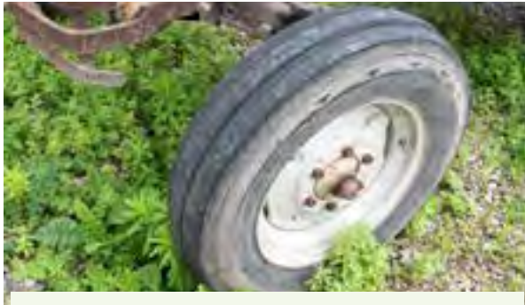
Fig. 4.6.5.b. Worn treads and dry rot make for poor traction and risk for downtime due to a blowout. Credit: Jeff Mathison
