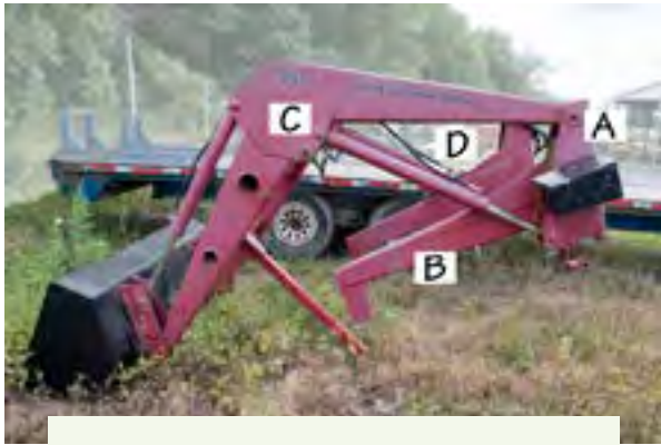
Figure 6.4.a. Front-end loaders may be parked and have to be mounted to the tractor you will operate. Components include: (A) The tower columns, which are hooked to the tractor's mid-frame and often serve as the support legs. Some smaller units may have a light duty rod that is inserted as the support leg. (B) Bar and saddle, which hooks to the tractor's front frame. (C) The lift arms and frame. (D) The hydraulic control system. Study the components before attempting to connect to the tractor. Tighten all connections securely. Credit: Jeff Mathison
