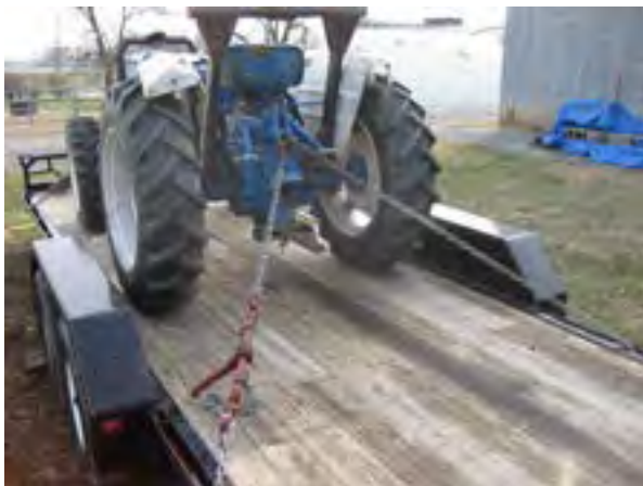
Figure 6.6.f. Secure the load (front and back) with straps or chains pointing down and outward. Credits: Penn State Extension Ag Safety Team and Michael Houtz, Penn State
