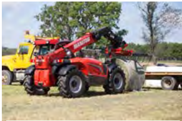
Figure 6.3.b. The telehandler load capacity chart must be used to determine if the weight of the round bales and the distance the boom must be extended to store them remains within the capacity range of the machine. Exceeding the weight and reach capacity of the telehandler could cause it to tip forward. Credit: Michael Houtz, Penn State
