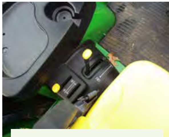
Figure 4.5.3.c. Some control levers may be left-side mounted. Credit: Penn State Extension Ag Safety Team
