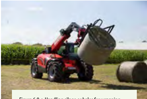
Figure 6.9.c. Handling silage or bales for wrapping may require a telehandler or tractor front-end loader. Be sure to follow safety practices. Travel with the load as low to the ground as possible. A heavy bucket of silage or bale will raise the machine's center of gravity as it is lifted. This will increase the risk of a tractor rollover. Credit: Michael Houtz, Penn State
