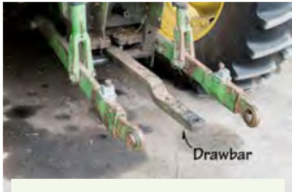
Figure 5.1.c. The tractor drawbar is the only safe place to connect a load. Do not hitch higher than the drawbar so all pulling forces stay below the tractor’s center of gravity. For most operations, the drawbar should be placed midpoint between the rear tires to maximize pulling power. Hillside operations may require a drawbar adjustment to one side to balance the pulling forces. Credit: Jeff Mathison
