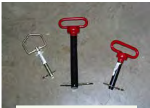
Figure 4.14.d. Secure hitch pins with locking clips as shown. Credit: Penn State Extension Ag Safety Team
