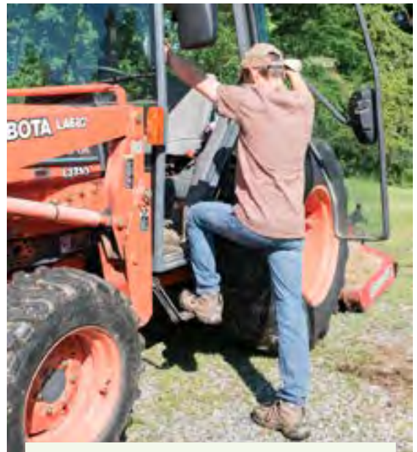
Figure 4.8.a. Mount a tractor safely by using the handholds and steps. Scraped shins, along with worse injuries, have occurred when handholds and footsteps are not used. Credit: Jeff Mathison
