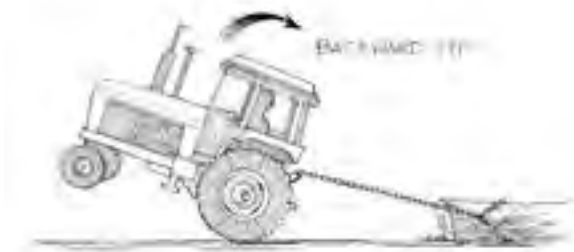
Figure 4.13.d. Hitch loads only to the drawbar. The drawbar has been engineered to pull heavy loads without risking a rear overturn hazard. Illustration by Jeff Mathison
