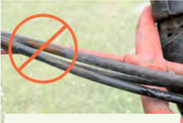
Figure 5.5.d. Hydraulic hoses may be reinforced, but damage to the outer covering—plus pinholes from high pressure—can cause serious injury (e.g., amputation) and machinery down time. Credit: Jeff Mathison
