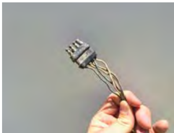
Figure 5.6.b. Grip the connector body to disconnect the wiring harness. Do not pull on the wires themselves. Become familiar with other connector styles before disconnecting them. Credit: Penn State Extension Ag Safety Team
