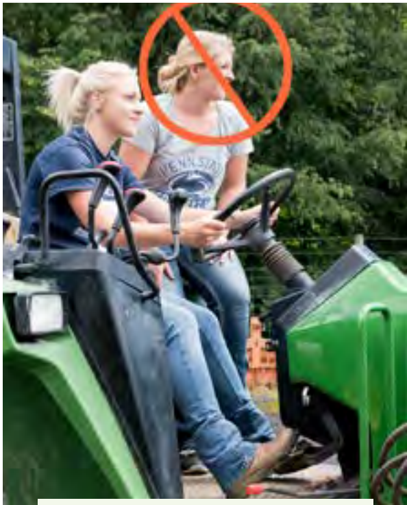
Figure 4.13.b. Tractors are designed for the operator only. No passengers allowed! Credit: Jeff Mathison
