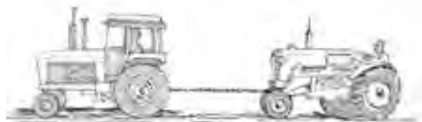
Figure 4.13.e. If you are stuck or need to be towed, you will need help. Specific tools are needed for this job. This is a job for adults only. A strap or chain may break, creating a hazardous situation. Illustration by Jeff Mathison
