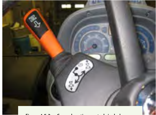
Figure 4.5.2.a. Ground motion controls include transmission controls, park-lock, and gear-shift levers. Credit: Penn State Extension Ag Safety Team
