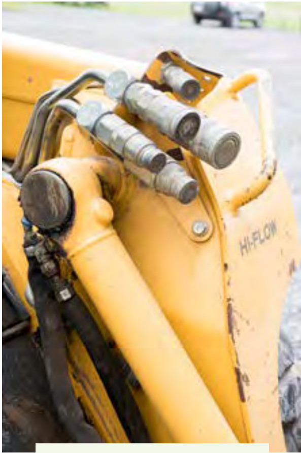
Figure 6.1.3.d. Hydraulic hoses are attached to the skid steer at conveniently located quick connection points. Credit: Jeff Mathison
