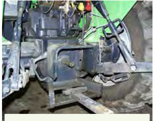
Figure 3.1.b. A PTO stub and a master shield on a tractor. A PTO is a wrap point hazard that causes countless injuries and deaths each year. Credit: Penn State Extension Ag Safety Team
