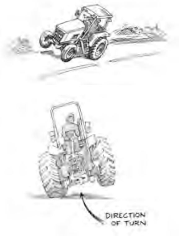
Figure 4.2.a. Tractor overturns can occur with high-speed sharp turns. Avoid sudden sharp movements in all tractor work. Illustrations by Jeff Mathison
