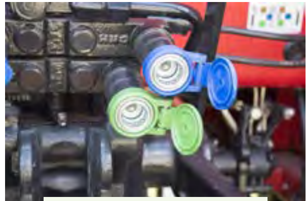
Figure 5.5.f. The female half of the hydraulic coupler is considered to be part of the tractor. Dust covers protect the quick release fitting, which includes the lock ring and ball lock mechanism. Credit: Jeff Mathison
