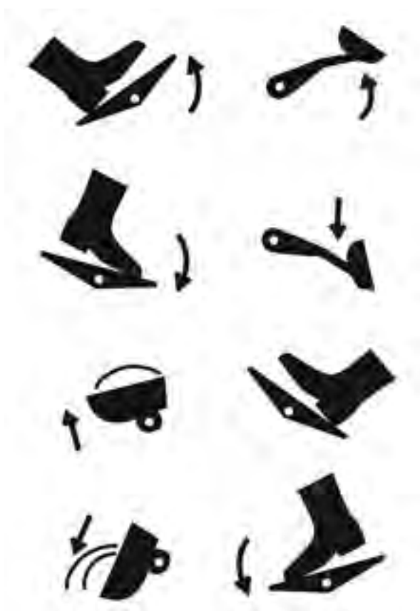
Figure 6.1.b. The hands and feet control the skid steer. Foot controls raise the lift arms (boom) and tilt or roll the bucket. The left heel raises the lift arms. The left toes lower the lift arms. The right heel rolls the bucket back to load. The right toes tilt the bucket to dump the contents of the bucket. Practice these actions before proceeding to operate the skid steer. Illustration by Jeff Mathison
