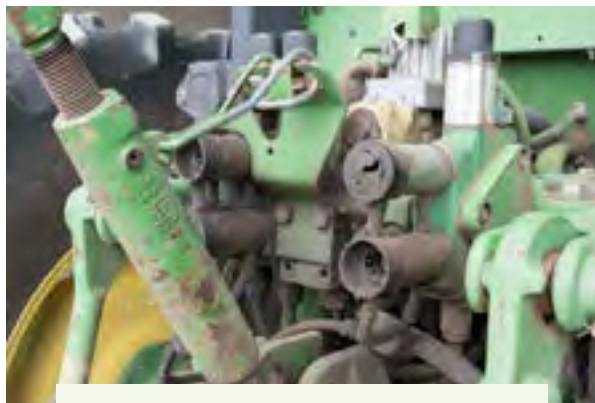
Figure 6.1.4.b. Missing hydraulic connection covers signify a problem in this picture. Credit: Jeff Mathison
