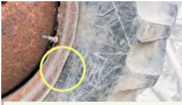
Fig. 4.6.5.c. Damaged rims from careless use may cause damaged tire beads and flat tires. Credit: Jeff Mathison
