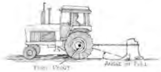
Figure 5.1.a. An example of safe hitching. The drawbar will lower if the front end lifts off the ground. This reduces the “angle of pull” and the risk of a rear overturn. Illustration by Jeff Mathison
