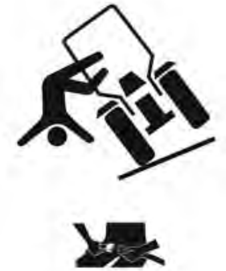
Figure 4.12.j. ROPS and a seat belt can protect you in the event of an overturn. If you are in the cab of a ROPS-equipped tractor, fasten the seat belt. Credit: Association of Equipment Managers
