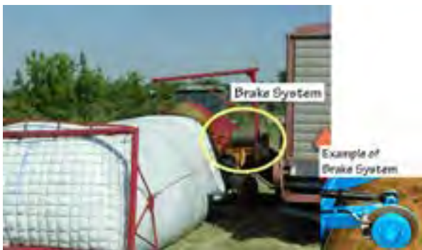
Figure 6.9.b. From the rear of the bagging equipment, the end-gate and cable braking system are shown. Large industrial disc brake(s) and a simple brake hand pump and brake pressure gauge control the rate of cable release. Silage bags may have convenient “stretch gauges” marked continuously along the bag to ensure packing consistency. Tension may be preset with experience or manually controlled during fill. Tension on the cable is released from the end-gate when the “bag” is filled. The end-gate can drop heavily to the ground. The close quarters between the wagon or truck being unloaded raise the potential for injury. Turning parts can snag loose clothes very quickly, and the tractor operator’s visibility of someone in this space is reduced. Credit: Penn State Extension Ag Safety Team
