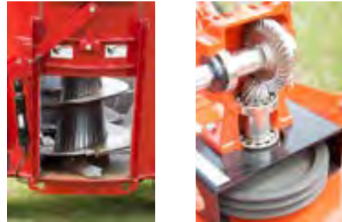
Figure 3.1.a. Pinch points can be found on most machines. Illustration credit: Association of Equipment Manufacturers; image credit: Michael Houtz, Penn State Extension.
