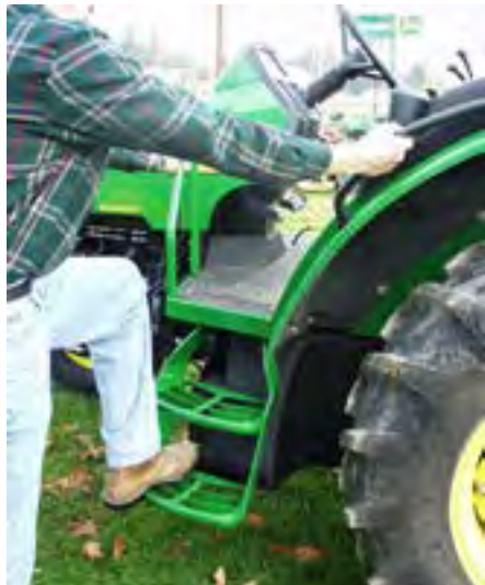
Figure 4.9.a. To prevent falls, use the handholds and footsteps provided to dismount from the tractor. Falls while dismounting account for many farm injuries each year. Credit: Penn State Extension Ag Safety Team
