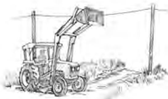
Figure 4.13.m. Avoid overhead power lines while transporting equipment to avoid risk of electrocution. Illustration by Jeff Mathison
