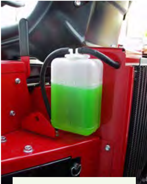
Fig. 4.6.1.d. Check the coolant level with the engine cold. Credit: Penn State Extension Ag Safety Team
