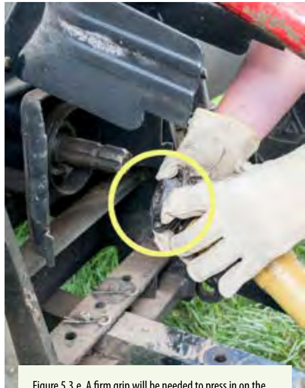
Figure 5.3.e. A firm grip will be needed to press in on the detent lock of the PTO shaft. This lock engages the groove in the stub shaft to secure the PTO driveline shaft to the stub shaft. See Task Sheet 5.4 for other forms of locking the PTO shaft. Credit: Jeff Mathison
