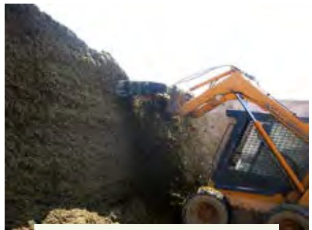
Figure 6.8.a. A hydraulic-powered, revolving-type silage defacer mounted to a material handler or skid steer is used to evenly remove the silage from the entire feed-out face of the silage. The construction of the defacer allows the operator to view the task easily. Credit: Jeff Mathison
