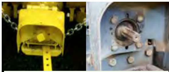
Figure 2.3.d. Be sure PTO shaft guards and stub shields are in place. Credit: Penn State Extension Ag Safety Team (shaft guards) and Jeff Mathison (stub shields)
