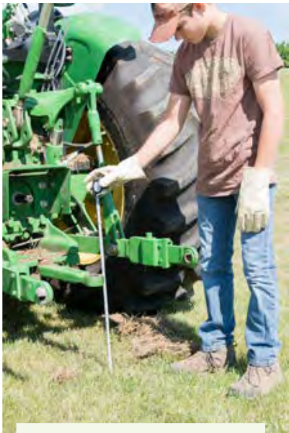
Figure 5.2.a. Taking a preliminary measurement of the drawbar height and the implement tongue before hitching makes aligning the two points much easier. A stable jack stand should be used to position the implement tongue. Always chock the wheels of the implement. Credit: Jeff Mathison
