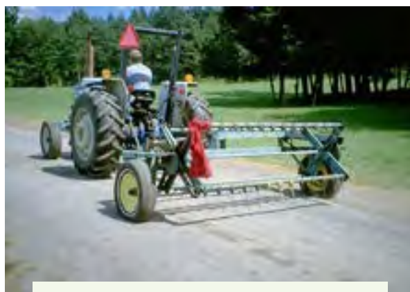
Figure 5.2.c. Implements can be wider than the tractor in transport or road position. Passing through farm gates or using public roadways can create a hazardous situation. Credit: Penn State Extension Ag Safety Team
