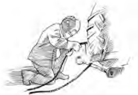
Figure 3.7.d. Welding sparks from electric arc welders and oxyacetylene gas welding equipment can create the spark that ignites nearby flammable materials or vapors. Illustration by Jeff Mathison
