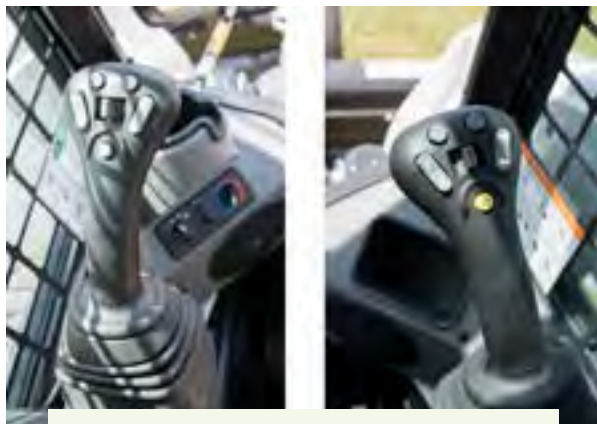
Figure 6.1.2.b. Joystick controls reduce operator fatigue. The joystick can be rotated to many positions and has fingertip button controls to move the skid steer, raise/lower lift arms, tip the bucket, and operate hydraulic-powered accessories. Credit: Jeff Mathison
