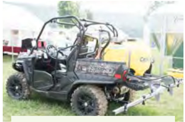
Figure 6.2.c. UTVs are versatile, allowing operators to do the smaller jobs that a pickup truck may be unsuited to do. Remember that the utility vehicle has limitations. Overloading, shifting loads, and sharp braking can cause turnovers. Credit: Jeff Mathison
