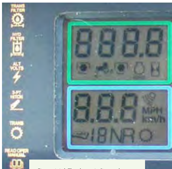
Figure 4.4.d. The charge indicator shows whether the alternator or generator is charging the battery properly. Credit: Penn State Extension Ag Safety Teams
