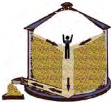
Figure 3.10.b. Grain flowing out of storage causes a downward-moving floor to move away from your feet. The victim is pulled waist deep in about 10 seconds. Credit: Penn State Extension Ag Safety Team
