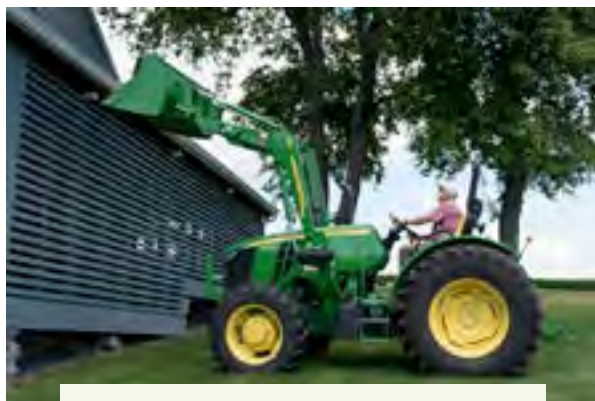
Figure 6.4.c. Extending the front-end loader with bucket or fork attachment moves bulky loads easily, but it also raises the tractor's center of gravity. This can allow the tractor to tip sideways more easily. Use the operator's manual to determine safe loading capacity. Credit: Jeff Mathison
