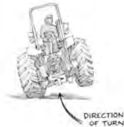
Figure 4.13.g. High speeds while making a turn can cause a sideways overturn. Make sure brakes are locked together. Reduce speed before entering the turn. Illustration by Jeff Mathison
