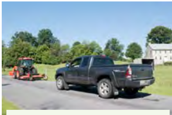
Figure 4.14.g. A best practice for transporting wide loads on a public roadway is to use an escort vehicle to assist in alerting other motorists. Be a courteous tractor operator to bring good public relations to the farm community. Credit: Jeff Mathison
