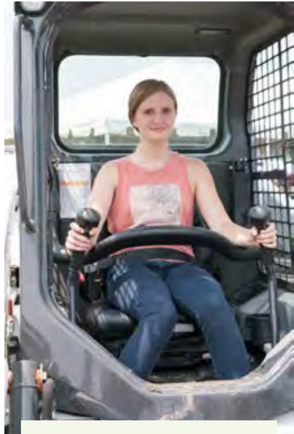
Figure 6.1.2.a. Control levers for moving or steering a skid steer are pushed forward, pulled back, or moved in some combination to “skid” the machine in the direction you wish to go. Notice the lap bar, which restrains the operator in the skid steer cab. Credit: Jeff Mathison
