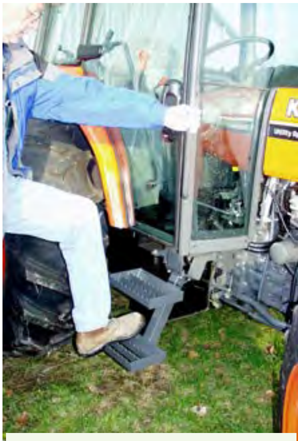
Figure 2.8.I. Use the handholds and face the steps when mounting the tractor. Credit: Penn State Extension Ag Safety Team
