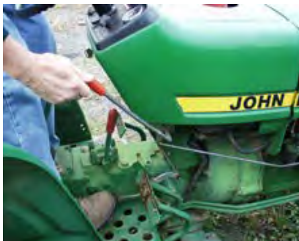
Figure 4.7.e. Set the throttle to 1/3 of its working range. Credit: Penn State Extension Ag Safety Team
