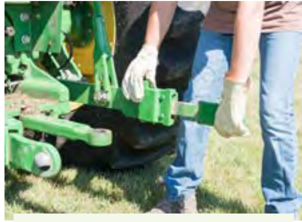
Figure 5.3.i. The telescopic extension to the draft arm is fully extended. In some cases, this must be done to align with the lower lift points of the three-point hitch implement. Be sure the extension is pushed back into the draft arm until locked into place when you are finished attaching the implement. Credit: Jeff Mathison
