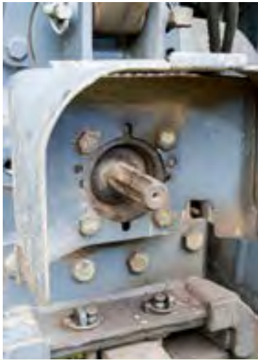
Figure 5.4.a. The 540-RPM PTO stub shaft has six splines (teeth) and is 1 3/8 inches in diameter. Credit: Jeff Mathison
