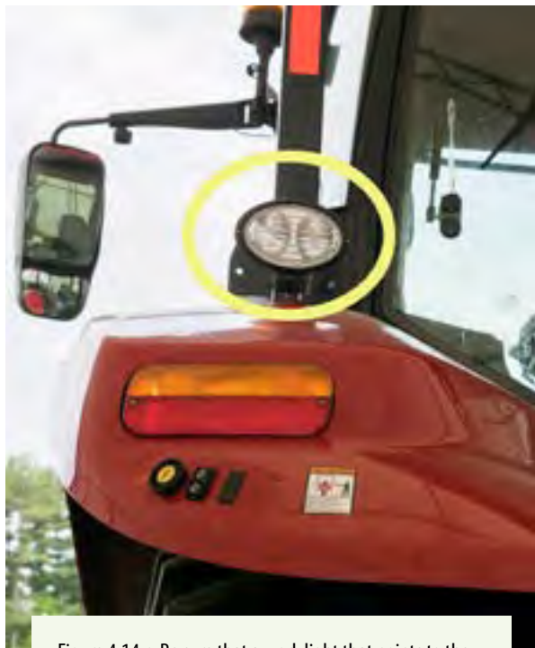
Figure 4.14.c. Be sure that a work light that points to the rear is off during road travel at night. Single white lights may not be recognized as slow-moving or as a tractor light. Replace SMV emblems that are worn, damaged, or faded. Credit: Jeff Mathison
