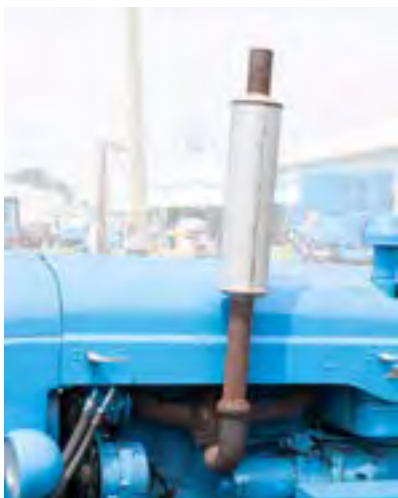
Figure 3.2.a. A straight pipe used for the exhaust or a worn-out muffler will increase noise levels coming from the engine. Muffler condition should be part of a safety audit. Credit: Jeff Mathison
