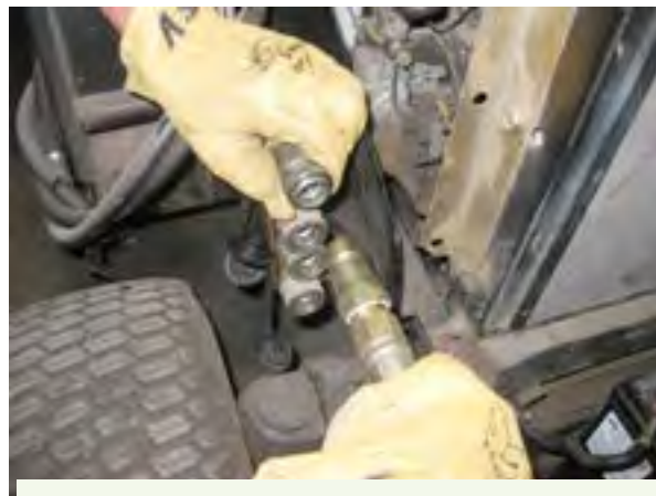
Figure 5.5.h. The lock ring of the female end of the coupling will secure the two fittings together. A firm grip will be needed to insert the hydraulic hoses from the implement (male end) into the coupling on the tractor (female end). Credit: Jeff Mathison
