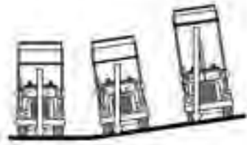
Figure 6.5.e. Raising the dump bed on sloped ground increases the risk of rollover. Longer trailers, windy conditions, and uneven loads add to the risk. Never attempt to unload a rig that is parked in a jack-knifed position. Illustration by Penn State Extension Ag Safety Team
