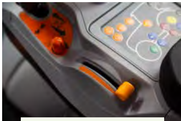
Figure 4.10.b. Remember that orange-colored control levers indicate ground motion controls. If the shift pattern is hard to locate, ask someone who is familiar with the tractor to show you the shift pattern. Credit: Michael Houtz, Penn State
