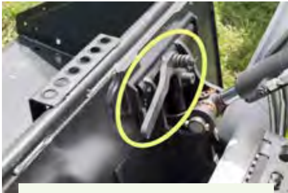
Figure 6.1.3.a. The standard latch handle lock for securing the attachment to the skid steer mounting plate is circled. The latch handle must be placed completely down to lock it in place. Credit: Jeff Mathison
