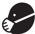
Figure 2.10.d. A NIOSH-approved dust mask is recommended when you see this symbol. Credit: AEM Pictorial Database
