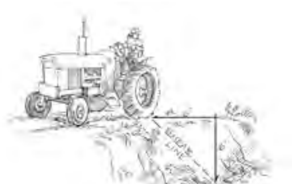
Figure 4.13.f. Avoid ditch embankments. Tractors are heavy and embankments can give way. For example, if the ditch is 6 feet deep, stay back at least 6 feet. Illustration by Jeff Mathison
