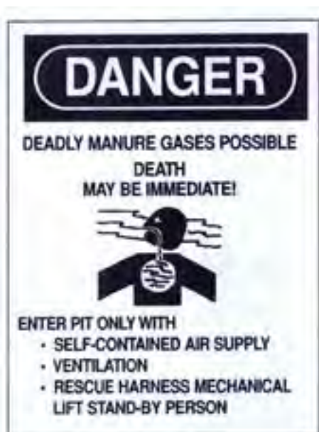
Figure 3.11.b. A danger sign posted near a manure storage structure provides a clear warning that immediate death is possible from manure gases. Credit: Penn State Extension Ag Safety Team
