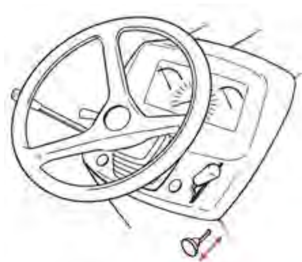
Figure 4.7.b. Choke the engine on cold days to allow more fuel than air to enter the combustion chamber. Release the choke after the engine has started—the fuel-rich mixture will foul the spark plugs and valves of the engine. Illustration by Andy Mylin
