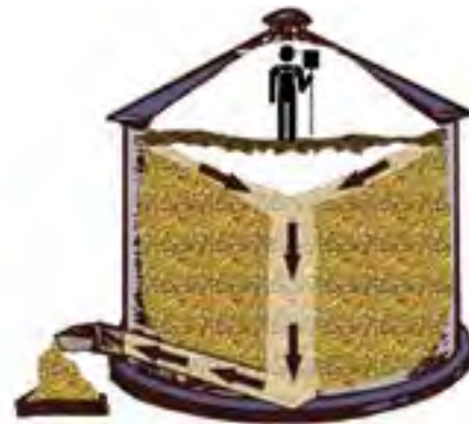
Figure 3.10.d. A "grain bridge" cannot support the weight of the worker. Credit: Penn State Extension Ag Safety Team
