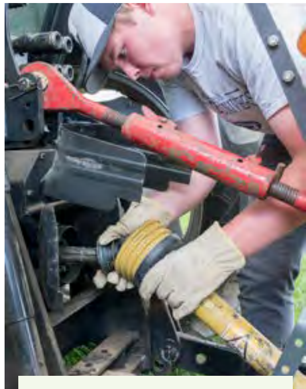
Figure 5.3.f. To attach the PTO shaft, you will be operating in a crowded space. Be sure the tractor engine is shut off and securely parked. Credit: Jeff Mathison
