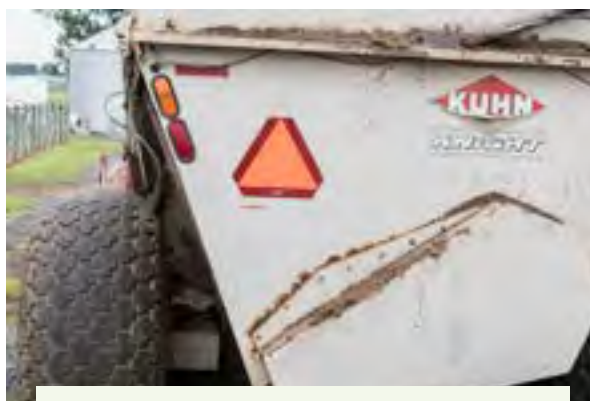
Figure 4.14.f. SMV emblems are required on vehicles designed to travel less than 25 mph while occupying public roadways. SMV emblems should be visible from no less than 1,000 feet to the rear of the tractor or towed implement. Therefore, mounting height may vary from 2 to 10 feet above the road surface. Replace faded, damaged SMV emblems. Newer tractors may need an SIS symbol as well. Credit: Jeff Mathison
