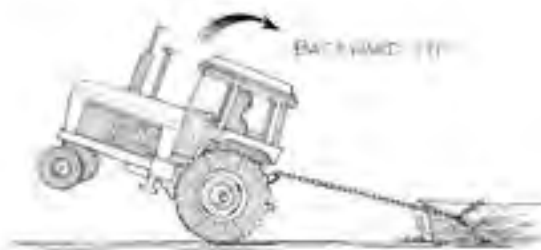
Figure 4.13.i. Tractors are powerful, but each one has a limit to its pulling power. Overloading a tractor could stall the engine, but rearward overturns can occur as well. Illustration by Jeff Mathison
