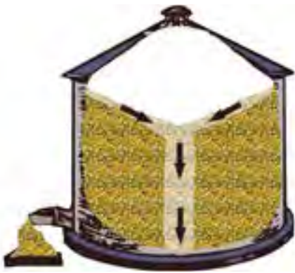
Figure 3.10.a. The normal flow of grain from a bin is off the top and down a center column of grain flowing toward the unloading auger. The unloading auger is found at the bottom center of the grain bin. Credit: Penn State Extension Ag Safety Team
