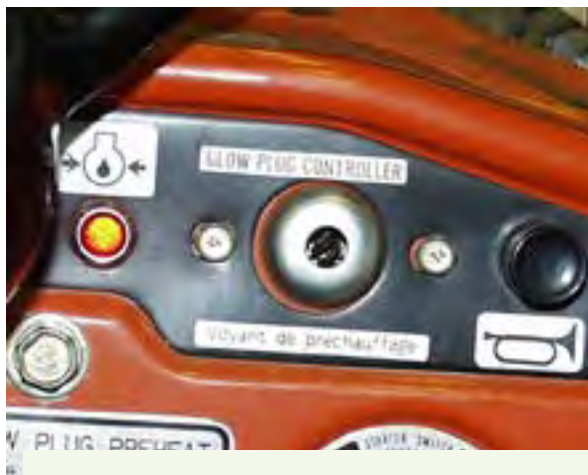
Figure 4.7.f. Turn the ignition key clockwise to the start position. Do not hold it there for extended periods of time. This can damage the starter motor or drain the battery of its charge. Credit: Penn State Extension Ag Safety Team
