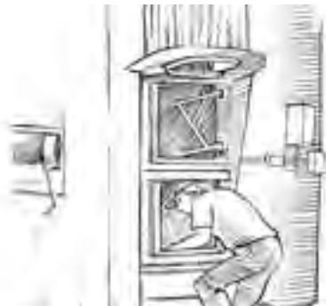
Figure 3.8.a. Confined spaces can kill! Never enter a confined space alone, and never enter if you are under the age of 16. Illustration by Jeff Mathison
