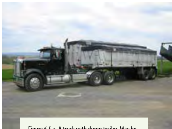
Figure 6.5.a. A truck with dump trailer. May be called a semi-trailer end-dump truck. Credit: Penn State Extension Ag Safety Team
