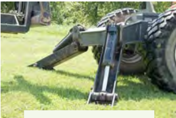
Figure 6.3.e. If the telehandler is equipped with outriggers use them to stabilize the machine during use. Credit: Jeff Mathison
