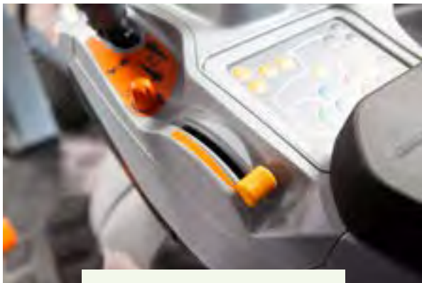
Figure 4.5.5.d. Engine speed control. Credit: Michael Houtz, Penn State
