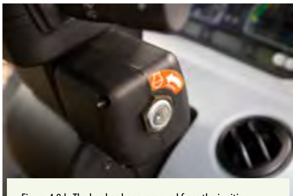
Figure 4.9.b. The key has been removed from the ignition. Untrained operators and children cannot start the tractor if the key is removed from the ignition. Michael Houtz, Penn State
