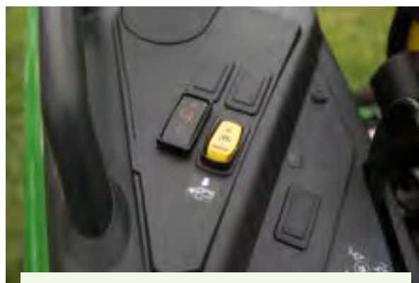
Figure 4.5.3.d. Rocker arm switches may be used. Credit: Michael Houtz, Penn State
