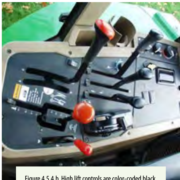
Figure 4.5.4.b. High lift controls are color-coded black. Credit: Penn State Extension Ag Safety Team
