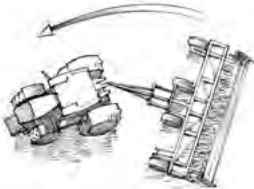
Figure 4.10.d. Too tight of a turning radius can damage tractor, tires, or implement. Illustration by Jeff Mathison
