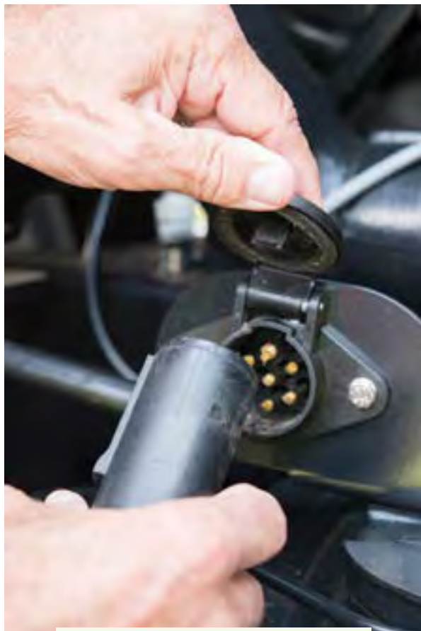
Figure 5.6.c. Align the pins of the electrical connection before attaching. Do not force the connector if the pins are not aligned. Threaded connectors do not pull loose; unscrew them first. Credit: Jeff Mathison
