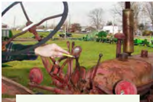
Figure 4.5.2.d. Older tractors may have the paint removed or were made before ground motion controls were color coded. Credit: Penn State Extension Ag Safety Team
