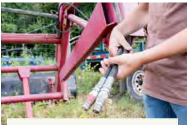
Figure 6.1.4.g. The male half of the coupler is part of the cylinder or hydraulic device system. Be sure to wipe dirt and grime from the hose end fitting. Credit: Jeff Mathison
