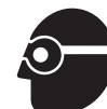
Figure 2.10.b. Goggles with impact-resistant lenses are recommended when you see this symbol. Credit: AEM Pictorial Database
