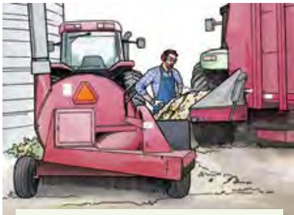
Figure 3.9.b. The work of filling a silo is done in close quarters. Two tractors are often involved, with the PTO shafts operating the self-unloading wagon and the silage blower. Extreme caution is needed to do this work safely. Credit: Andy Mylin
