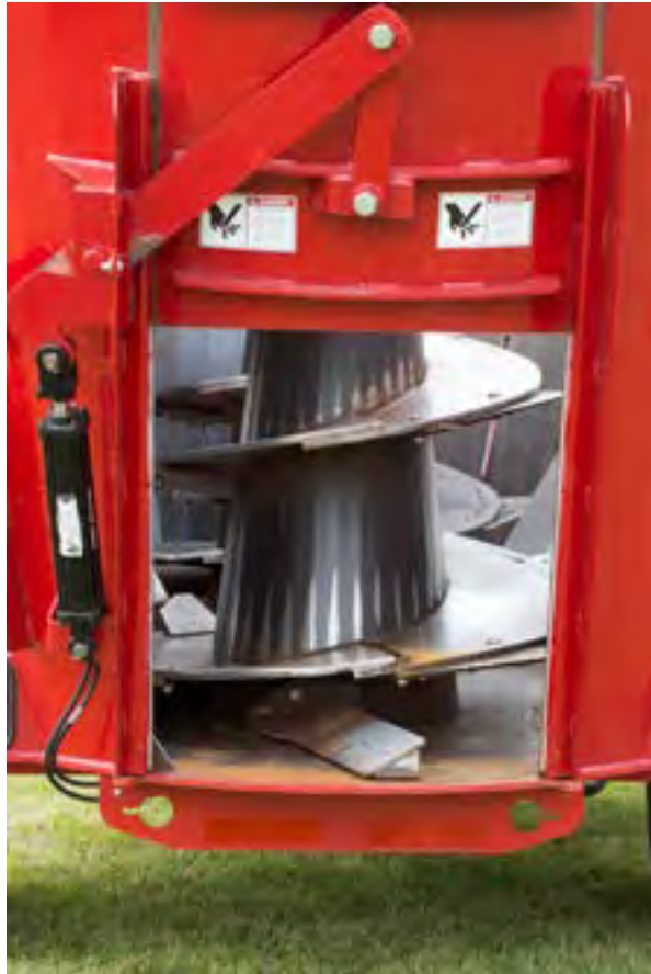
Figure 6.7.d. A total mix ration (TMR) mixing wagon loads from the top by high-lift bucket. This is not a normal work position and because the distance away from the operator is considered to be guarded by location. (A hazard is “guarded by location” when it is guarded by other parts or components of the machine that are not themselves guards or when the hazard is beyond the safety distance. The high sides of the mixer wagon form a “barrier” to prevent the hazardous area from being reached inadvertently.) DO NOT ENTER this mixing space that has three augers moving close together. Credit: Michael Houtz, Penn State
