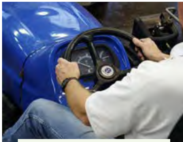
Figure 4.10.c. Use both hands to steer the tractor. If you hit a hole in the field, the wheel can be jerked from your hand. Credit: Penn State Extension Ag Safety Team
