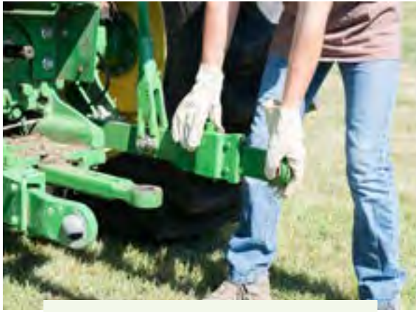
Figure 5.3.h. If the three-point hitch is equipped with an extension to the lower draft arm, release the lock and pull or extend the draft arm extension to the rear before nearing the implement to be attached. Credit: Jeff Mathison
