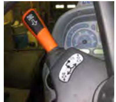
Figure 4.10.2.b. Look on the left side of the steering column. The shuttle shift lever, sometimes called the reverser, allows for ease of changing direction without using the clutch. This lever may serve as the positive park to be used with the parking brake. Some may have to be in a neutral position for the tractor to start. This may be the only time that the clutch pedal is used. Credit: Penn State Extension Ag Safety Team
