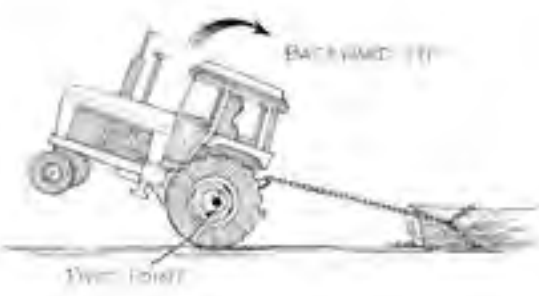
Figure 5.1.b. The log is fairly immovable. A chain hooked above the center of gravity of the tractor (e.g., top of three-point hitch bracket) allows a rearward tip of the tractor. Improper hitching has overridden safe tractor engineering design. Many people have lost their lives as a result. Illustration by Jeff Mathison
