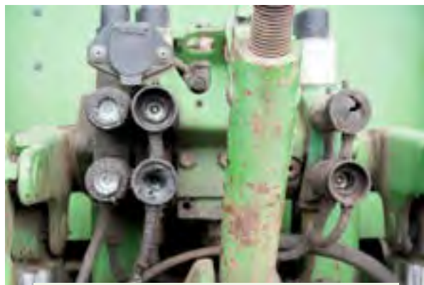
Figure 5.5.b. Missing hydraulic connection covers signify a problem with this tractor. What will happen to the hydraulic system if the dust covers are not kept in place? Credit: Jeff Mathison
