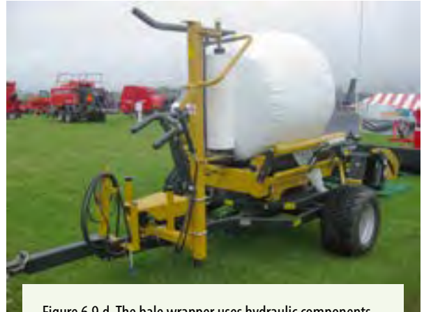
Figure 6.9.d. The bale wrapper uses hydraulic components to rotate the bale in two directions to wrap the plastic film snugly. Once covered, a shear arm cuts the plastic, the bale is dropped to the ground, and another bale lifted into place for wrapping. Since this is done from the tractor seat, the operator is physically removed from machine hazards. Keep children and bystanders away from the wrapping operation. Credit: Penn State Extension Ag Safety Team
