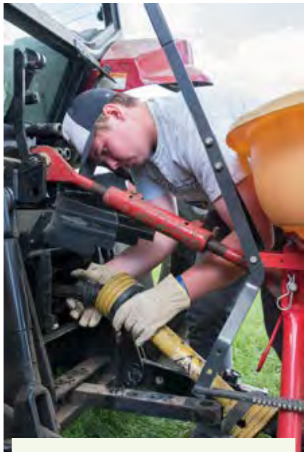
Figure 5.4.g. This is what the task of connecting a PTO looks like. You must lift a heavy object at an awkward angle while squeezing in the lock mechanism detent pin. Watch someone else connect a PTO several times before doing this job. Continue practicing connecting a PTO on your own with supervision. Credit: Jeff Mathison
