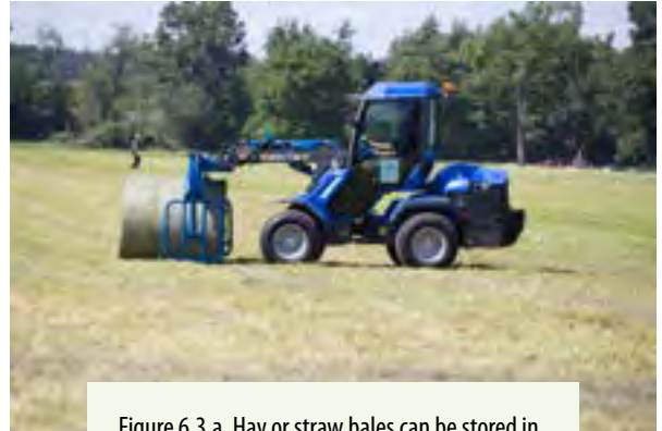
Figure 6.3.a. Hay or straw bales can be stored in an area that requires the use of a telehandler. Credit: Michael Houtz, Penn State
