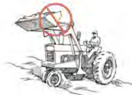
Figure 4.13.k. When operating a high-lift bucket with a load or without a load, keep the bucket as low to the ground as possible while in transport. Sideway overturns are possible if you try to travel with the bucket in the up position. Illustration by Jeff Mathison
