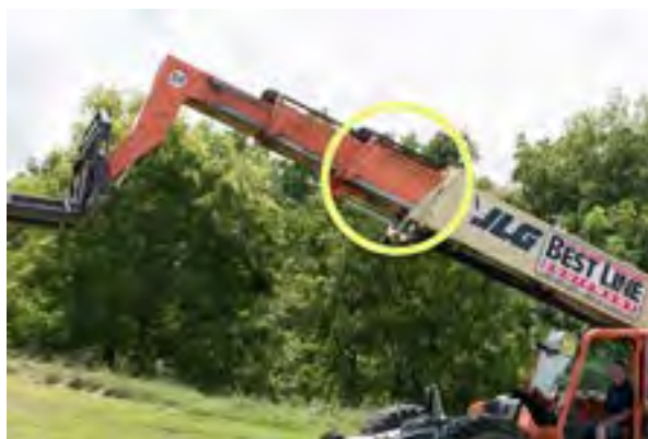
Figure 6.3.c. As the boom is extended a letter (circled) or number markings are revealed that are referenced in the operator's cab to give restrictions on how much weight can be lifted safely. A boom angle indicator is included. Credit: Jeff Mathison
