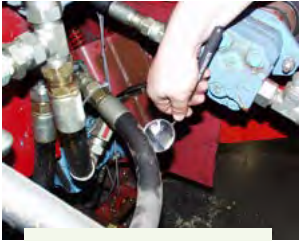
Figure 6.1.4.e. Use a mirror or piece of cardboard to check for high-pressure hydraulic leaks. Do not use your hand! Pinhole leaks are often invisible. Credit: Penn State Extension Ag Safety Team
