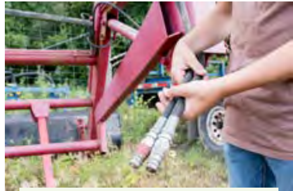
Figure 5.5.g. The male half of the coupler is part of the cylinder or hydraulic device system. Be sure to wipe dirt and grime from the hose end fitting. Credit: Jeff Mathison
