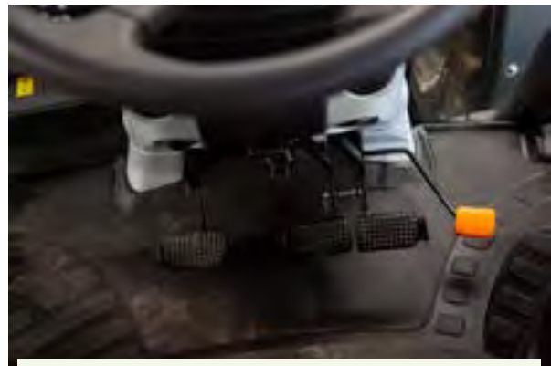
Figure 4.5.5.c. Clutch control. Credit: Michael Houtz, Penn State
