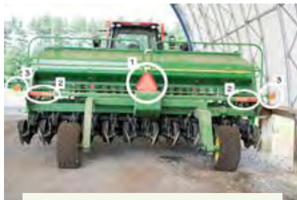
Figure 4.14.1.b. Lighting and marking features used on this tractor and grain drill: number 1 is the SMV, number 2 shows hazard and signal lights, and number 3 is the conspicuity material as a red retro-reflective marker. Credit: Jeff Mathison
