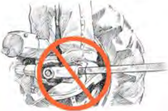
Figure 2.3.a. Never step across a turning PTO shaft. Loose clothing can be pulled into the shaft before you are able to react. Illustration by Jeff Mathison
