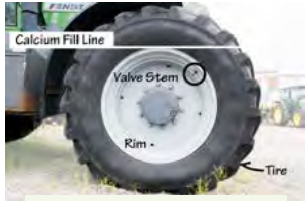
Figure 4.6.5.a. Tractor tire components may include the tire, the rim, an inner tube with a valve, and, many times, a liquid solution filling the inner tube to serve as a liquid ballast. Credit: Jeff Mathison
