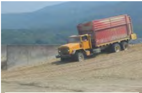
Figure 3.9.1.d. Dump trucks are commonly used to fill horizontal silos. A truck equipped with a webbed unloading floor is more stable than a raised-bed truck. Operate the truck up and over the drive-over pile, not across the slope, and up and then down on a trench fill silo. Credit: Penn State Extension Ag Safety Team
