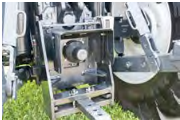
Figure 5.4.h. This PTO stub shaft is protected with a tractor master shield and stub shaft cover. To remove the stub shaft cover, grip the cover firmly and turn counterclockwise. Store the stub shaft cover where it will be available to replace when the job is done. Credit: Jeff Mathison
