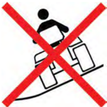
Figure 6.2.d. Avoid steep banks. Utility vehicles can easily overturn. The driver must know the machine and the work area to reduce potential risk of injury. Credit: Association of Equipment Manufacturers
