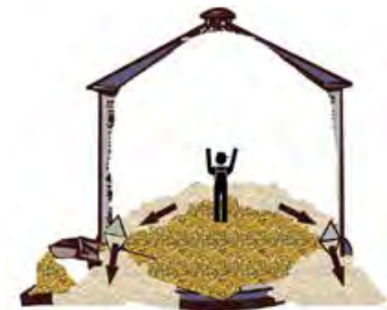
Figure 3.10.g. It takes much force to remove a victim of grain bin entrapment. Rather than removing the victim, it is easier to remove the grain. Special tools and skills are needed to cut through grain bins and remove the grain. Credit: Penn State Extension Ag Safety Team
