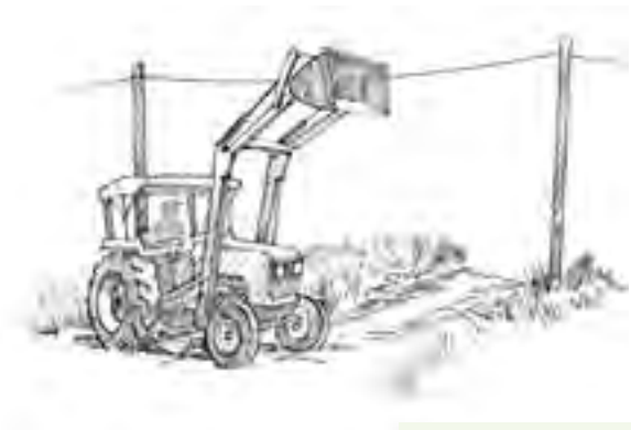
Figure 6.4.d. To prevent electrocution, lower the front-end loader bucket to avoid power lines crossing the work area. Illustrations by Jeff Mathison
