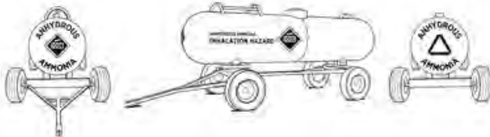
Figure 3.12.b. Anhydrous ammonia tanks must be plainly marked on all surfaces as containing an inhalation hazard. Such markings provide the message that this material is deadly. Illustrations by Andy Mylin
