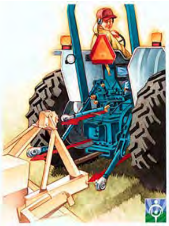
Figure 5.3.a. Back slowly to the implement to be attached. Using the hydraulic controls, raise or lower the draft arms to nearly match the implement's lower hitch pins. Credit: Youth Work Guidelines
