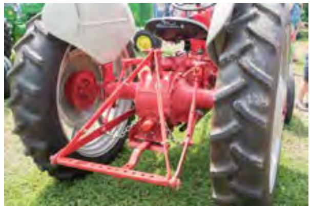
Figure 4.12.h. Never hitch to the top link of a three-point hitch. Credit: Jeff Mathison
