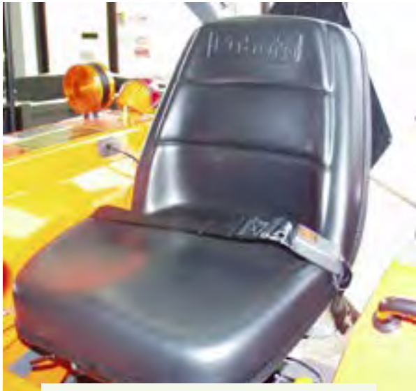
Figure 4.6.6.c. Tractors with ROPS come equipped with seat belts. Use them. Credit: Penn State Extension Ag Safety Team
