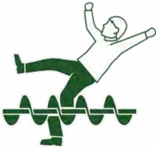
Figure 6.7.b. Missing auger guards and shields increase the risk for injury or fatality. Your employer must provide a safe workplace. Credit: Agricultural Youth Work Guidelines
