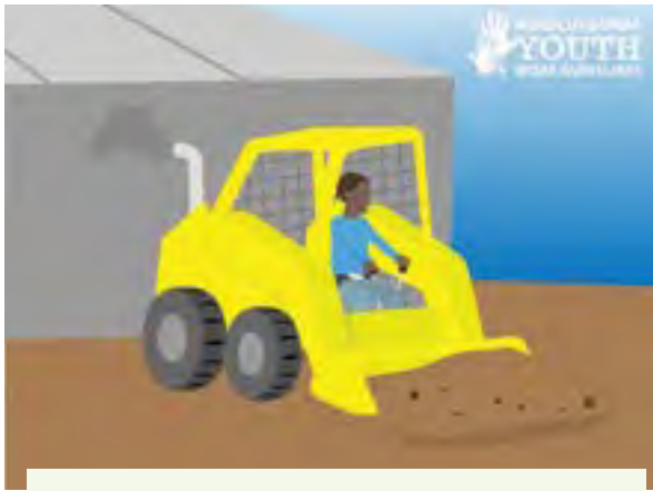
Figure 1.2.2.b. OSHA regulations specifically cover ROPS, seat belts, and guarding of moving machinery parts. Be responsible and know what is required. Credit: NAGCAT
