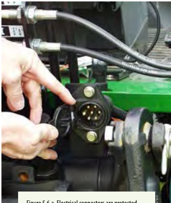
Figure 5.6.a. Electrical connectors are protected from dust, dirt, grease, and grime with dust caps. Keep these covers repaired and in place to ensure electrical connections can be made without delay. Credit: Penn State Extension Ag Safety Team
