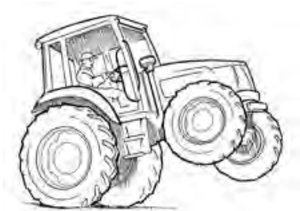
Figure 4.10.a. Start the tractor moving smoothly. Excessive engine speed can cause the tractor to start with a jerk. Illustration by Andy Mylin
