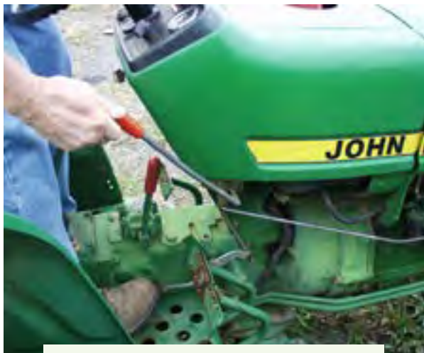
Figure 4.5.1.b. Diesel engines are often stopped by shutting off the fuel flow from the fuel pump. Credit: Penn State Extension Ag Safety Team
