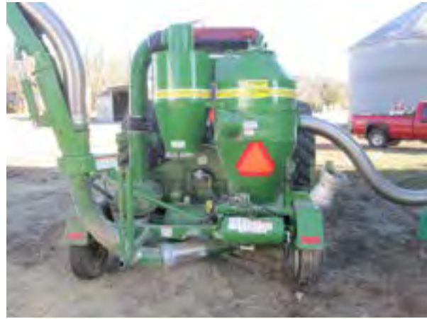
Fig.3.10.h The grain vacuum moves large quantities of grain from storage to truck, or from truck to grain bin. Credit: Jeff Mathison
