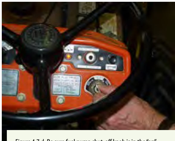
Figure 4.7.d. Be sure fuel pump shut-off knob is in the "on" position. If the conditions are cold, turn the ignition key to the glow-plug setting and hold until the indicator shows that the combustion chamber is hot enough to ignite the diesel fuel droplets. If you don't know how to do this, ask someone to show you. Credit: Penn State Extension Ag Safety Team
