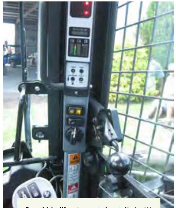
Figure 6.1.1.a. When the operator is seated in the skid steer seat with seat belt fastened or operator restraint bar in place, the instrument panel lights will indicate that system functions are ready to use. Credit: Penn State Extension Ag Safety Team
