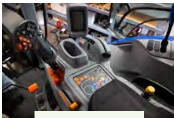
Figure 4.5.5.f. Ground speed control. Credit: Michael Houtz, Penn State
