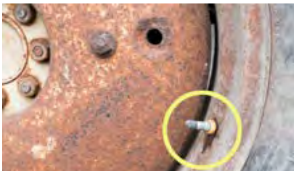
Fig. 4.6.5.d. A leaking valve stem released calcium solution, which rusted the rim. A major expense will be incurred, and using this tractor presents a severe safety hazard. Credit: Jeff Mathison
