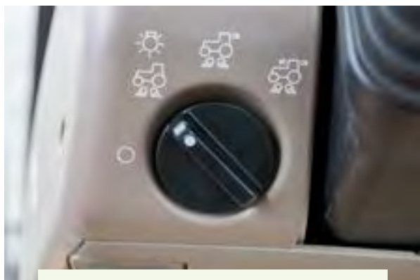
Figure 4.5.4.c. The light control switch is a black rocker switch. Credit: Jeff Mathison
