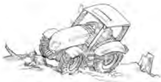
Figure 4.13.h. Avoid obstacles as you operate the tractor. Some tractor operators will check the field before beginning the operation. Stumps, rocks, animal dens, etc., can upset a tractor. Illustration by Jeff Mathison
