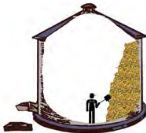
Figure 3.10.f. Damp, moldy grain can stick to the side of the grain bin. It can collapse on the worker who tries to dislodge it. Credit: Penn State Extension Ag Safety Team
