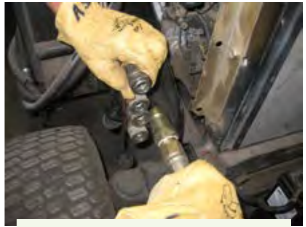
Figure 6.1.4.i. A firm grip will be needed to insert the hydraulic hoses from the implement (male end) into the coupling on the tractor (female end). Credit: Penn State Extension Ag Safety Team
