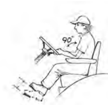
Figure 4.6.6.f. The steering wheel should be adjusted as soon as you are seated. In the correct position, your arms are bent at a 90-degree angle as you hold the steering wheel. Your legs should remain slightly angled while the foot pedals are fully depressed. Credit: Jeff Mathison
