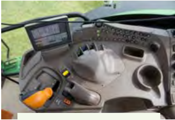
Figure 4.10.2.c. Visual monitoring of speed and power ranges are made to assist the operator in efficient operation. Someone must explain the system to you so that you can operate the tractor properly. Credit: Michael Houtz, Penn State
