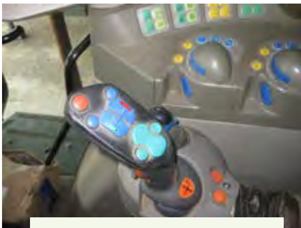
Figure 4.10.2.e. Tractor's imported into the United States may not use the same color-coding standards for controls as tractors manufactured for the U.S. market. Request training before using imported tractors. Credit: Penn State Extension Ag Safety Team
