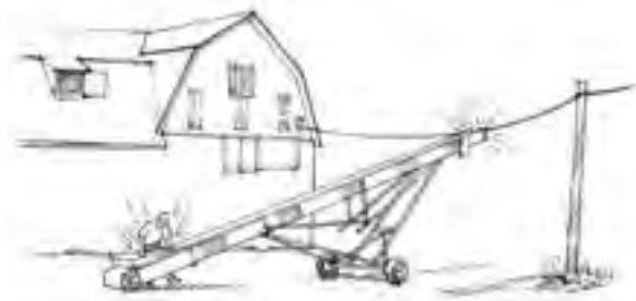
Figure 3.6.b Lower the hay elevator or grain auger to avoid contact with overhead power lines. Illustration by Jeff Mathison
