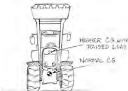
Figure 4.12.d. A raised CG makes it easier for a tractor to turn over sideways. Illustration by Jeff Mathison
