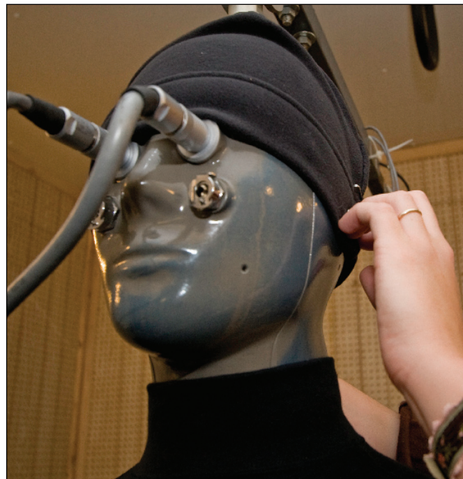
Meet Stan , an integral member of Professor Elizabeth McCullough's research team. STAN is equipped to measure just how well a piece of winter clothing protects its wearer from the cold.
