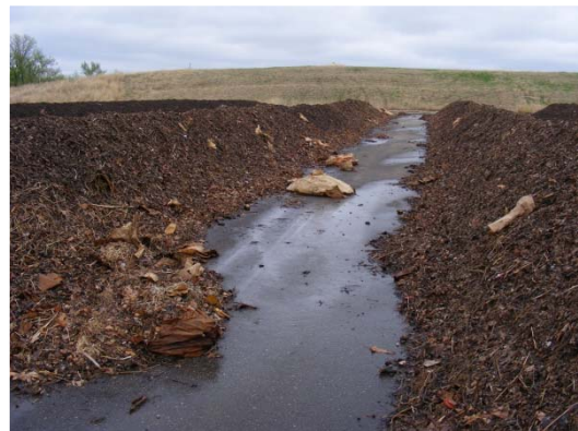
Figure 1: Two distinct windrows are seen piled high. These piles are limited by the width of the turner that will be used to aerate the compost pile. Mechanized aerators are used to mix fresh oxygen into the compost pile to maintain aerobic decomposition.
