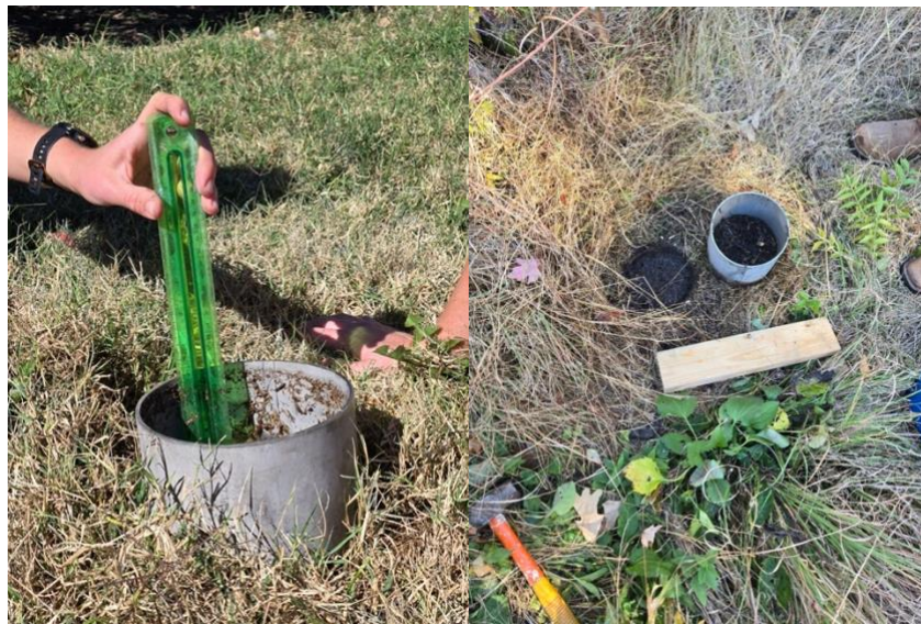
Fig. 2 – A) Shows the water depth measurement in the infiltration ring. B) Shows the cleared testing spot and the tools used to insert the infiltration ring.
