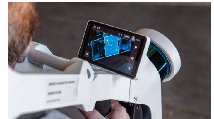
Tom Harris, an engineer with TDI, straps on the NavVis system and step-by-step scans the second floor of the building in Jetmore, Kansas.
